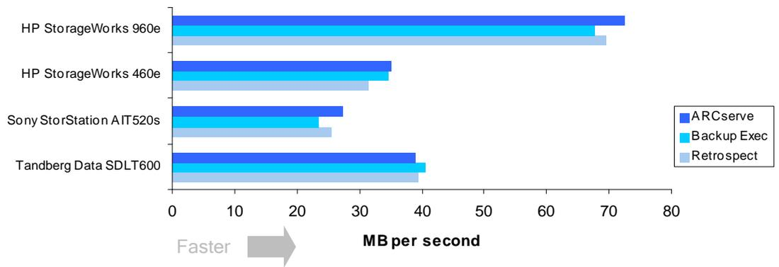
In general, all three products returned similar results for the data restoration tests although ARCserve, once, again proved to be marginally faster than the rest. With the HP StorageWorks Ultrium 960, ARCserve returned 72.4MB/sec which was 4 per cent faster than Retrospect and 7 per cent faster than Backup Exec. The smallest margins came with the Tandberg Data SDLT600 with all three products returning restoration speeds of between 39MB/sec and 40.5MB/sec.
