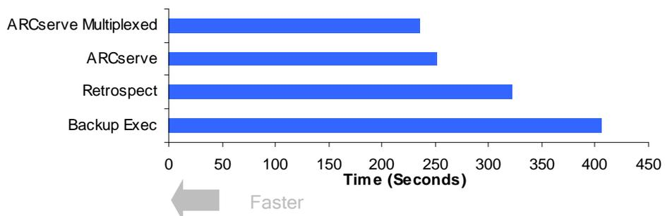
As can be seen from the test results ARCserve's multiplexing feature delivers clear performance advantages when backing up clients over the network. Comparing results from the sequential backup and multiplexed tasks for ARCserve alone show a 41 per cent improvement with the tasks taking 646 seconds and 382 seconds respectively.
