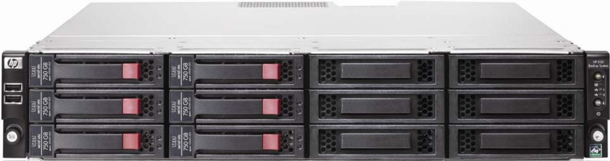
HP is currently offering two solutions for the SME market with the family comprising the D2D2500 and the D2D4000 featured in this report. The D2D4000 is a 2U rack mount appliance with room at the front for up to twelve drives with the 4.5TB model under test sporting six 750GB SATA hard disks mounted in the same sturdy hot-swap carriers as used across a wide range of HP's servers and storage appliances.
