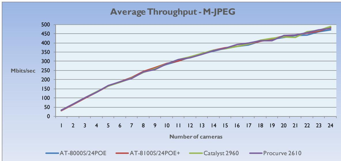
The higher demand for network bandwidth of M-JPEG video streams can be seen clearly in the above graph. Furthermore, as we increased the number of video streams we found that the system running the Axis Camera Station Network was having increased difficulty in playing each one correctly.
