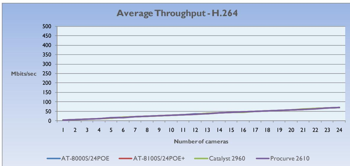
Comparing the two throughput graphs shows the dramatically reduced network requirements for the H.264 video streams. For each switch, the average throughput measured for all 24 streams was between 68Mbits/sec and 70Mbits/sec as opposed to 472Mbits/sec to 479Mbits/sec for M-JPEG.
