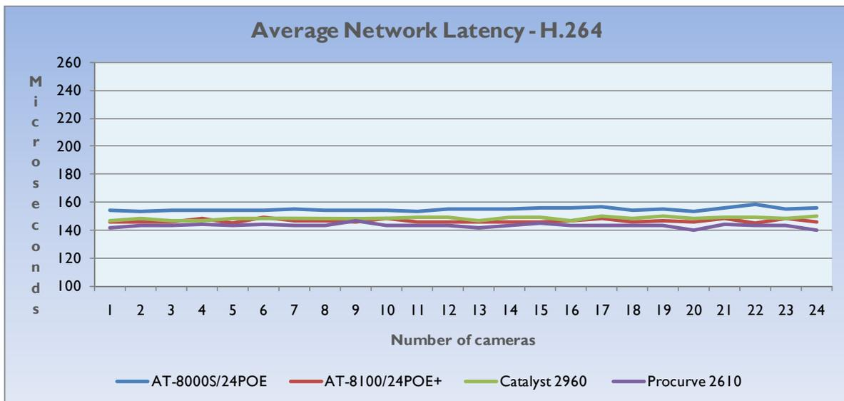
The effects of the lower network bandwidth requirements for H.264 are also reflected in the latency tests. Unlike the M-JPEG tests where latency gradually increased, we found that the H.264 streams showed no increase in latency regardless of the number of camera feeds.
