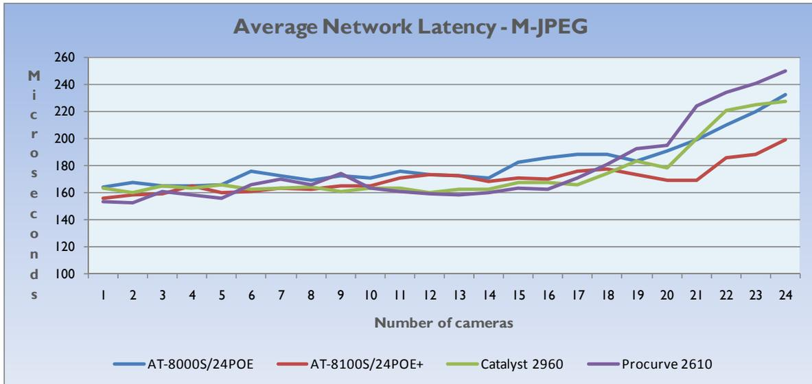
It should be noted that these results show the time taken in microseconds (millionths of seconds) for a data packet to traverse the network and not just the switch backplane. For the M-JPEG test, network latency is slightly higher than for the H.264 feeds at the beginning but as the load increases it gradually gets worse for all switches. However, we did find that the AT-8100S/24POE+ switch consistently delivered the lowest latencies for this test.
